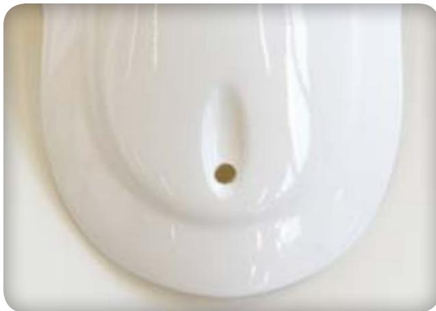
Drill a 8mm hole in your canopy and glue the grommet holder in place.
