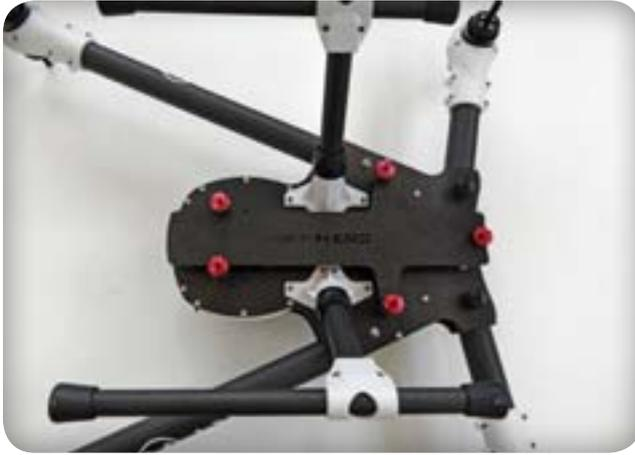
Screw the quick release nut on landing gear holder and slide legs into it.
