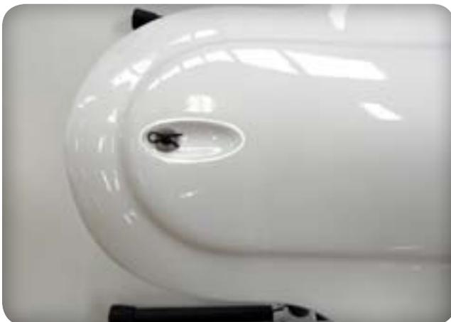
Mount the grommet into holder, fix the canopy with the body clip.
